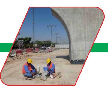
Field density test (FDT) to ensure the compaction
