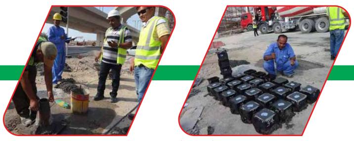
Testing at site: checking of Workability (Slump test), Concrete cubes making
