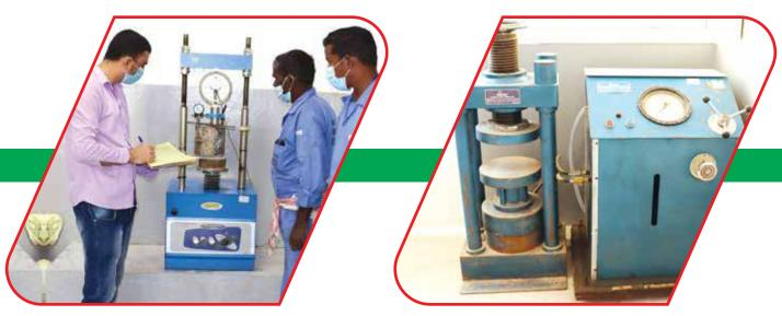
Testing at laboratory: checking of cube compressive strength
